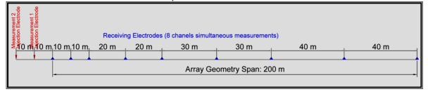
Array geometry for D30B and D30C sector: pole-dipole
