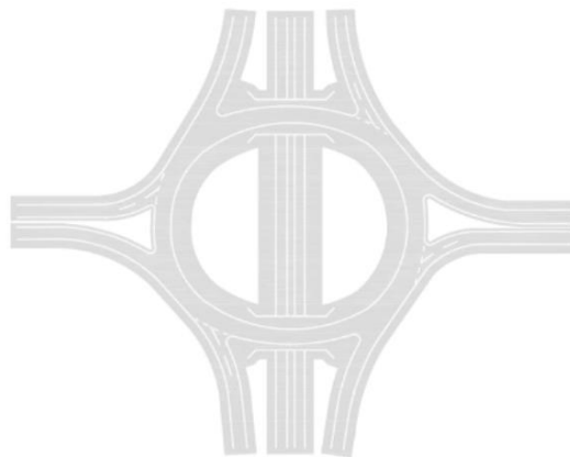
Figure 11 - Extract from UK DMRB CD122. Geometric Design of Grade Separated Junctions – Two Bridge Junction
